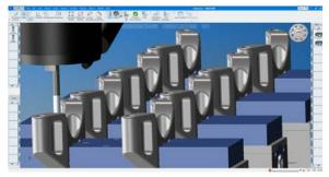
Multiple part setups are easily defined, giving users the ability to increase part production and reduce programming time.
